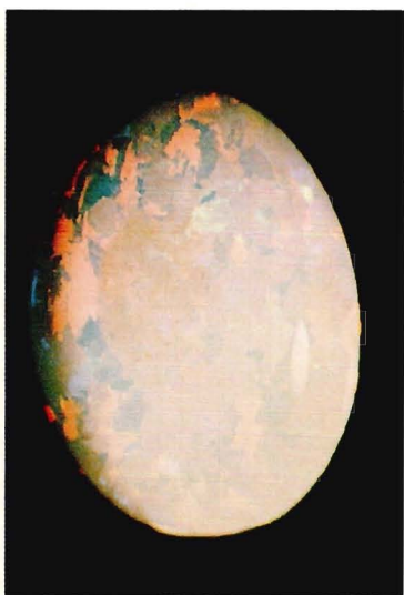
FIG. 5. Synthetic white opal (Gilson, Sept. 1975) showing broadly "equigranular" texture, overall milkiness, and turbid central patch. \times 5 reflected light.
