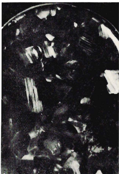
FIG. 15. Natural opal, showing mosaic with some "albite twinning" structures. \times 7.5 reflected light.
