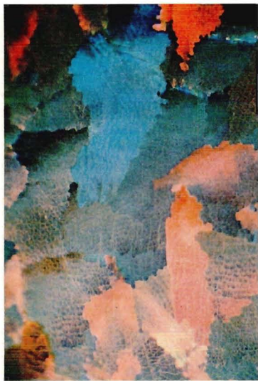
FIG. 14. Synthetic black opal (Gilson, Dec. 1975) showing "lizard skin" effect and crenulate margins. \times 12 , reflected light.
