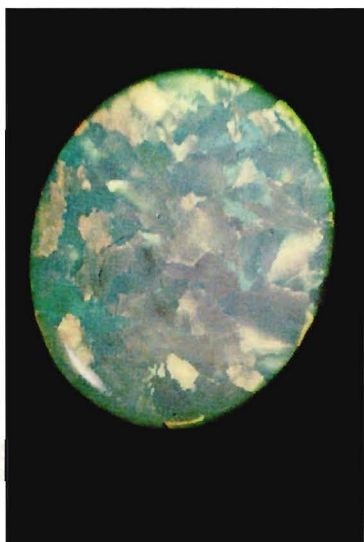
FIG. 11. Synthetic white opal (Gilson, Nov. 1975) showing mosaic, "lizard skin" effect and overall iridescence in yellow-green. \times 4 , reflected light.
